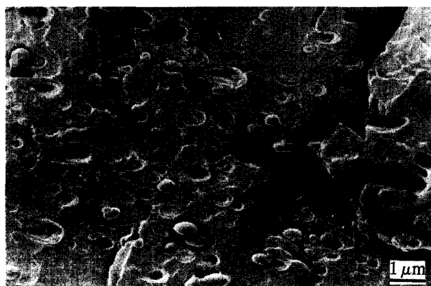
Figure 8 SEM of a cryo-fractured 10/90 LDPE/PVC blend, compatibilized by 1.0 wt% of EBSAN-20 (processed in a micro-extruder)
