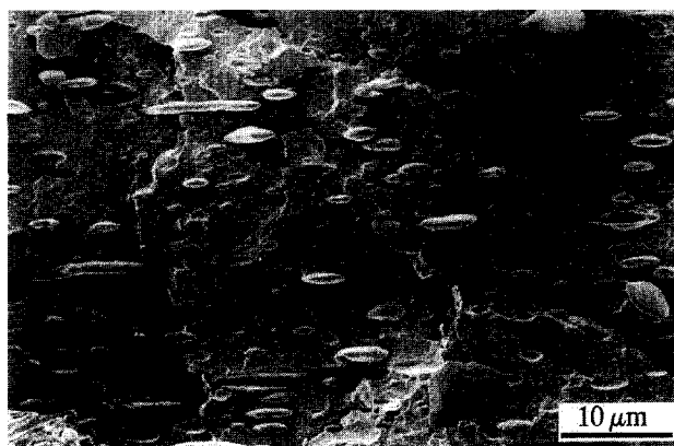
Figure 4 SEM of a cryo-fractured 10/90 LDPE/PVC blend (processed in a micro-extruder)
